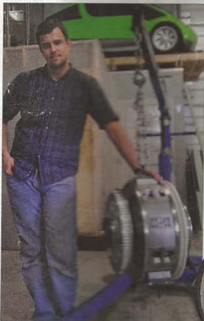
The Niama-Reisser NR-1 concept car holds four passengers, weighs 1,200 pounds, and is reported to get 200 mpg at 70 mph. The car's 7.0L Centrifugal Heinz Boxer (CHB) engine represents a clean break from traditional combustion engines. The CHB engine uses a pair of opposing torus-shaped pistons (they look like a section of a doughnut) that oscillate in a rotary motion. Torque is applied to the crankshaft with a mechanism that can also vary the compression ratio (beyond 25:1).
