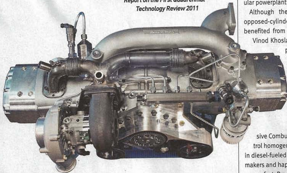
EcoMotors is located in Allen Park, Michigan. Its EM100 is a two-stroke, opposed-piston, opposed-cylinder turbodiesel. The cylinder bore is 3.937 inches and the engine weighs 296 pounds. The engine measures 22.8x41.3x18.5 inches and is rated for 325 hp at 3,500 rpm while torque is 664 lb-ft at 2,100 rpm.
